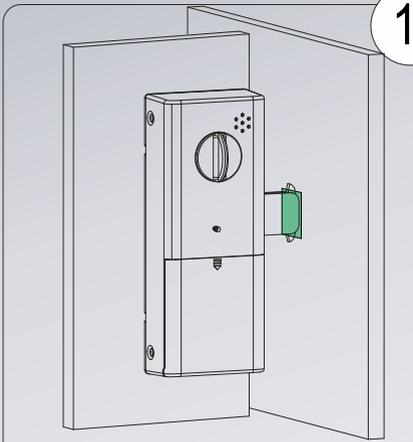
Install the main lock (installation method is the same as above), and then unscrew the lock tongue to mark it when the door is closed naturally.
