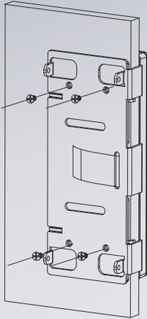
Firstly push the U clip from the side of the glass door and screw up 4 fixing screws.
