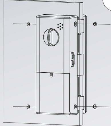
Plug in the cables and cover the back panel and then screw up 4 fixing screws.
