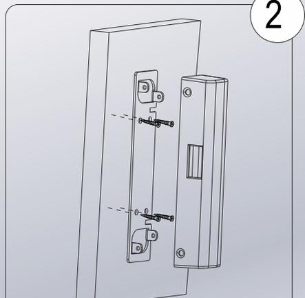
The side lock should be fixed directly with self tapping screws or rivet and also the back panel should be fixed with screws.
