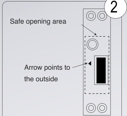
Note: When the blade is installed, its triangle direction must point to the outside (the hole should be opened according to the size of opening drawing)
